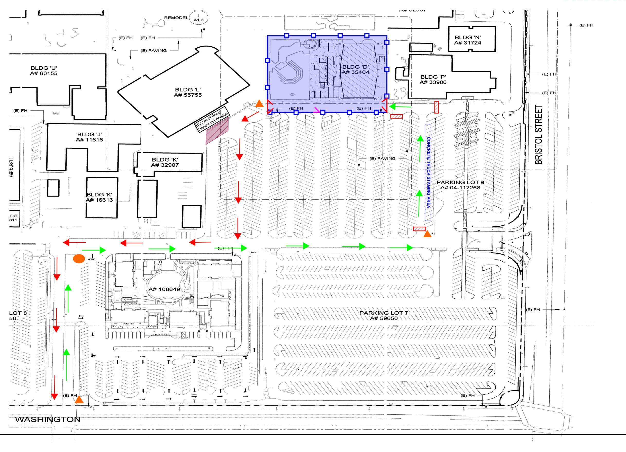
Concrete Truck Route (IN)——Concrete Truck Route (OUT)——Construction Entrance/ \ \ Man Gates \ \ Flagman \ \ Directional Sign
